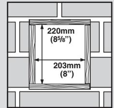
After constructing tunnel, proceed to step 6b.
